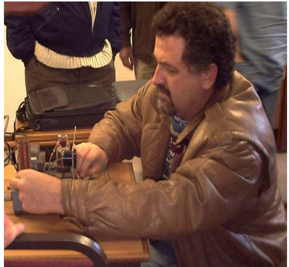
Following Bill, Wynand ZS6ARF surprised us with a 6146 valve QRP rig that he demonstrated to be capable of 15 W maximum. The photo below shows him giving it a tune-up with Almero ZS6LDP looking on.
